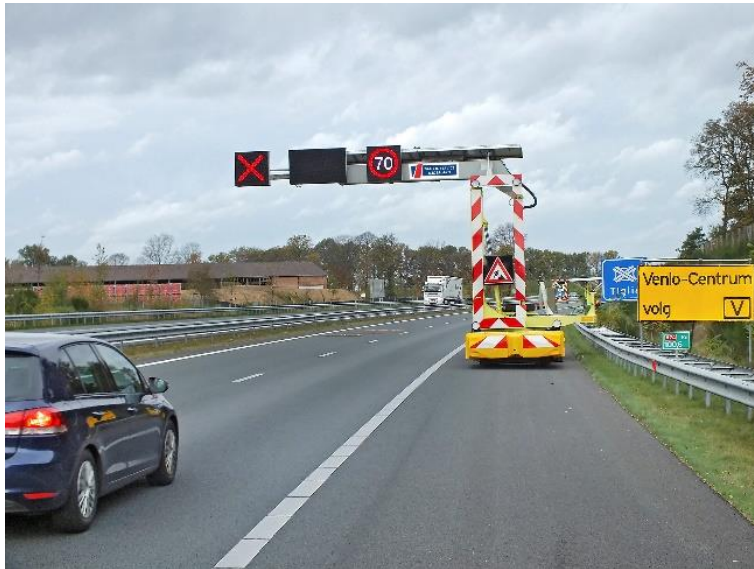
Figure 11: Example of Mobile Gantry Crane
